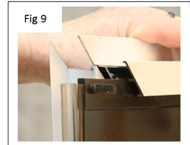
Install the new flap with textured side facing out. Align the side of the frame and attach with the screw that was just removed.
